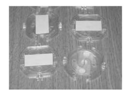
This case deals with socket protectors. These are devices that users (parents) put into the electrical socket outlets to stop small children from accessing live parts by putting a long metal object into one of the holes in the outlet and getting a (fatal) electric shock.
